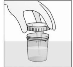
**Moving the sample to vacuum tube**
